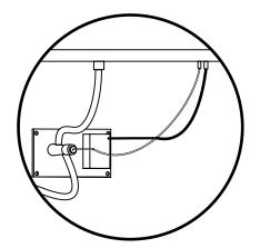
• Ensure the black wire from the system is connected to the igniter.
