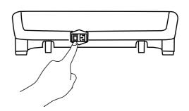
X If the rollers get stuck, turn off the switch and press the ON/OFF button, the roller will be back to its initial position.
